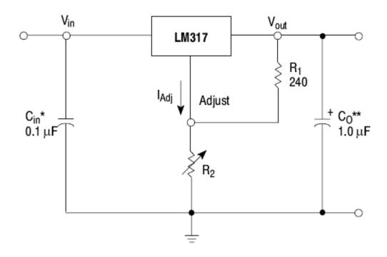
Note A: Use of an input bypass capacitor is recommended if regulator is far from filter capacitors.
